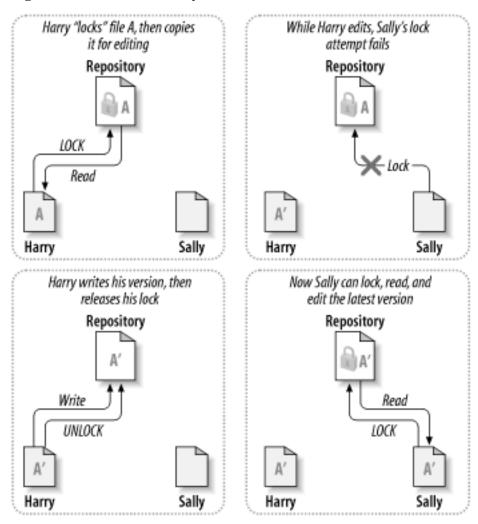
Figure 2.3. The lock-modify-unlock solution
