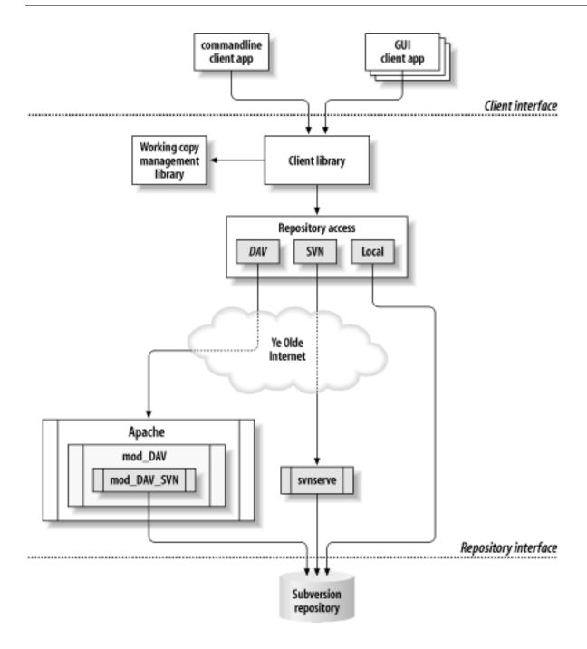
On one end is a Subversion repository that holds all of your versioned data. On the other end is your Subversion client program, which manages local reflections of portions of that versioned data (called "working copies"). Between these extremes are multiple routes through various Repository Access (RA) layers. Some of these routes go across computer networks and through network servers which then access the repository. Others bypass the network altogether and access the repository directly.
